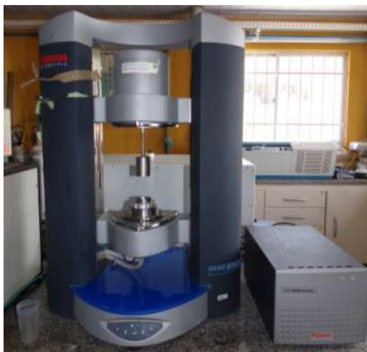
Figura 15 – Reômetro Haack Maars.
