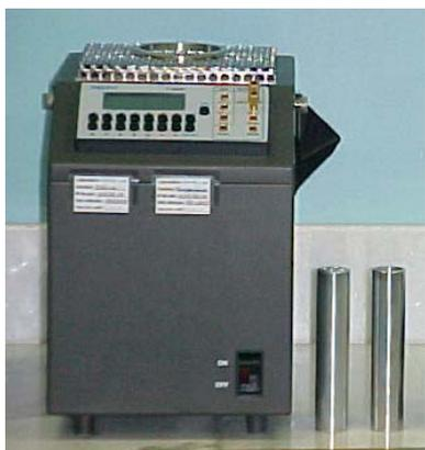
Figura 12 – Calibrador Presys (T-350P)
