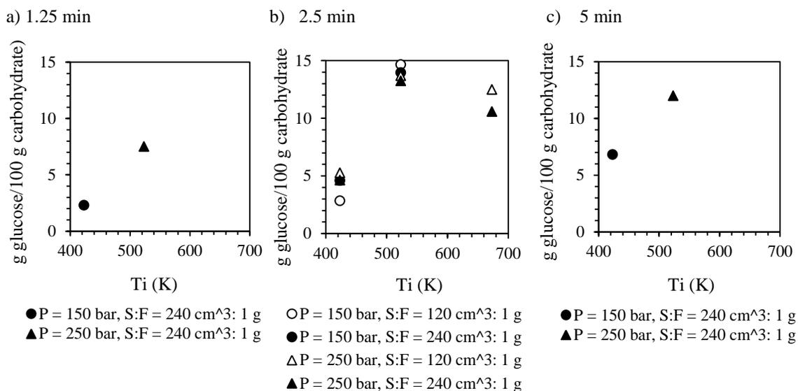
**Figure 3.** Total reducing sugar yield of hydrolyzate fractions for subcritical hydrolysis of defatted pressed palm fiber for residence time of a) 1.25 min, b) 2.5 min and c) 5 min
