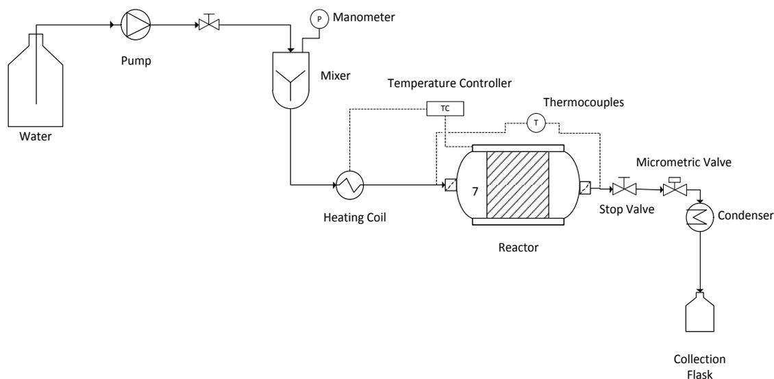
**Figure 1.** Scheme of the subcritical water hydrolysis unit.
